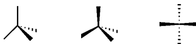
Figure 2-68. Different possibilities for the display of stereochemistry; the one in the middle is not unambiguous and therefore is not allowed.
